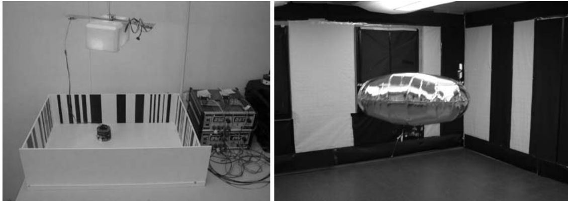
Figure 2.1: Evolutionary vision-based robots. Left : The Khepera equipped with a linear camera (16 pixels, 36^\circ FOV) was positioned in an arena with randomly sized black and white stripes. Random size was used to prevent development of trivial solutions whereby the controller would use the size of the stripes to measure distance from walls and self-motion. Right : The blimp-like flying robot, provided with a similar linear camera (16 pixels, 150^\circ FOV), is closed in a 5 \times 5 \times 3 m room with randomly sized black and white stripes on the walls.
